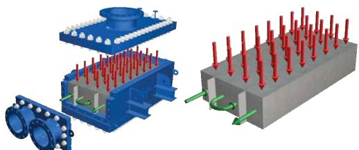
Single pass tube system in combination with corrugated side sandwich system for multiphase applications (e.g. condensation)
