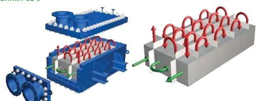
High number of passes tube side system in combination with corrugated side sandwich system for close temperature approach applications (heat recovery)
