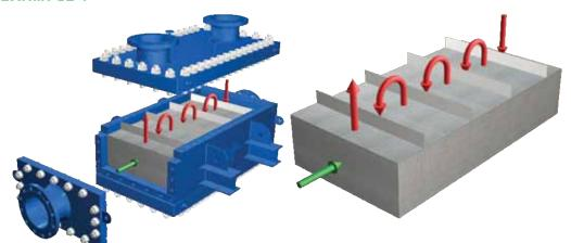
Low number of passes tube side system in combination with single pass corrugated side system for low NTU value applications and/or low pressure drop requirements
